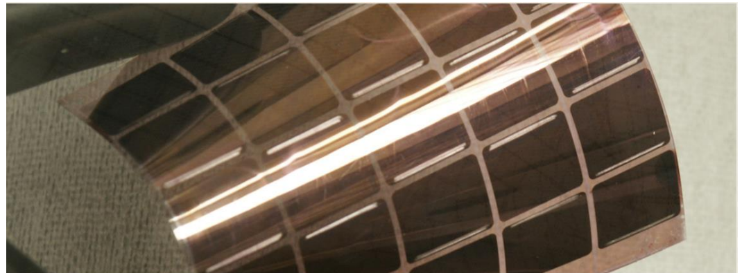
Flexible photovoltaic module based on organic semiconductors
